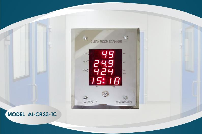
The CLEAN ROOM SCANNER is micro controller based indicator for indicating clean room differential pressure, temperature & humidity with synchronized high accuracy clock. This instrument has been designed mainly to monitor any 3 process parameters using external analog inputs from third party transmitters including temperature, %R.H., and Diff. pressure as standard & optionally any other analog input from front end transmitters for indoor air quality, CO, CO2 & air velocity, etc.
