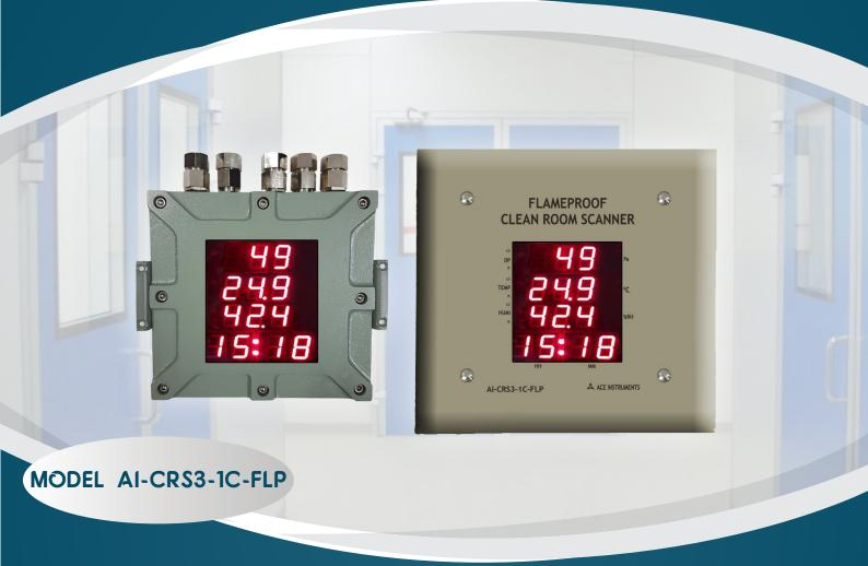
The FLAMEPROOF CLEAN ROOM SCANNER is micro controller based indicator for indicating clean room differential pressure, temperature & humidity with synchronized high accuracy clock. This instrument has been designed mainly to monitor any 3 process parameters using external analog inputs from third party transmitters including temperature, %R.H., and Diff. pressure, indoor air quality, CO & air velocity transmitter, etc.
